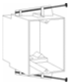
Single gang, 18 inches 3 Work box Captive mounting nails. Two Quick Click® entries for each end. 2.0625" W x 2.875" H x 3.125" D (52.4 x 73.1 x 79.4 mm). 4oz (.1kg) 7200-450075: S1-18-R
